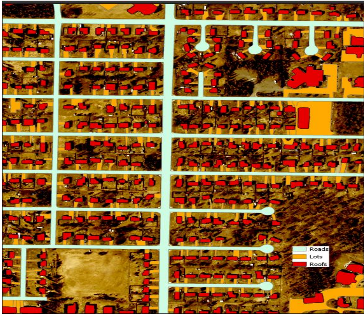
Figure 4. Example of Completed Impervious Surface Mapping.
