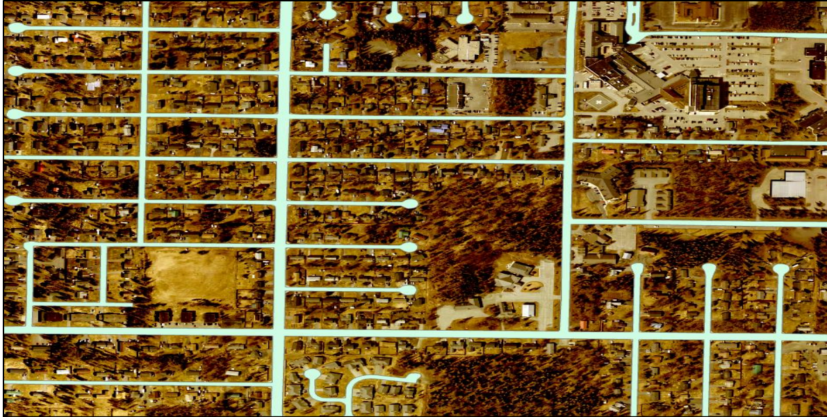
Figure 3. Snippet of Output of Roads Extraction Tool Buffered.
