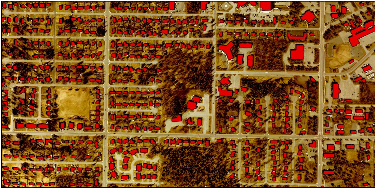
Figure 2. Example of Output of Detect Objects Using Deep Learning Module Using the Extract Building Footprints Model.
