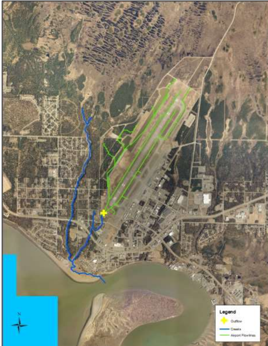
Figure 4. The portions of the flow network that run off the Kenai Airport are in green.
