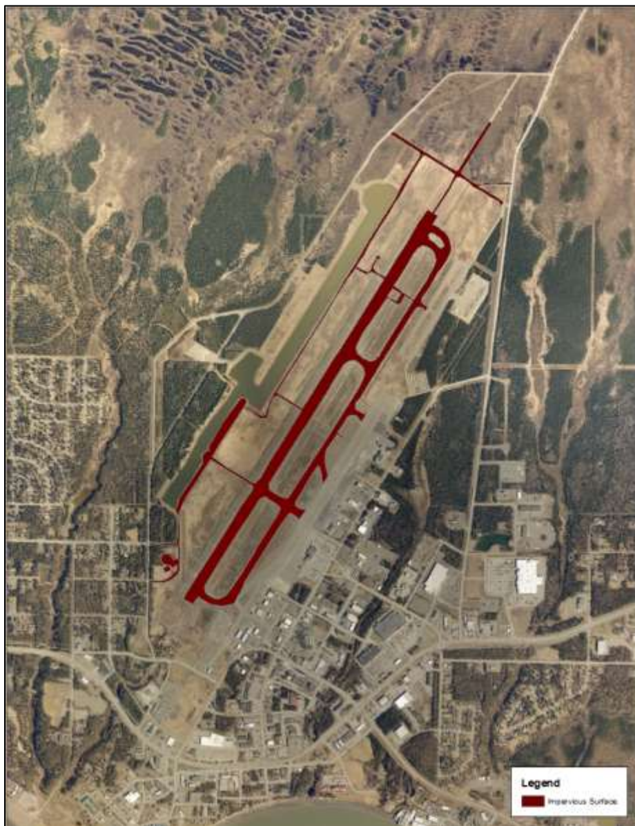
Figure 5. Impervious surface where flow direction is to the southwest culvert outlet.
