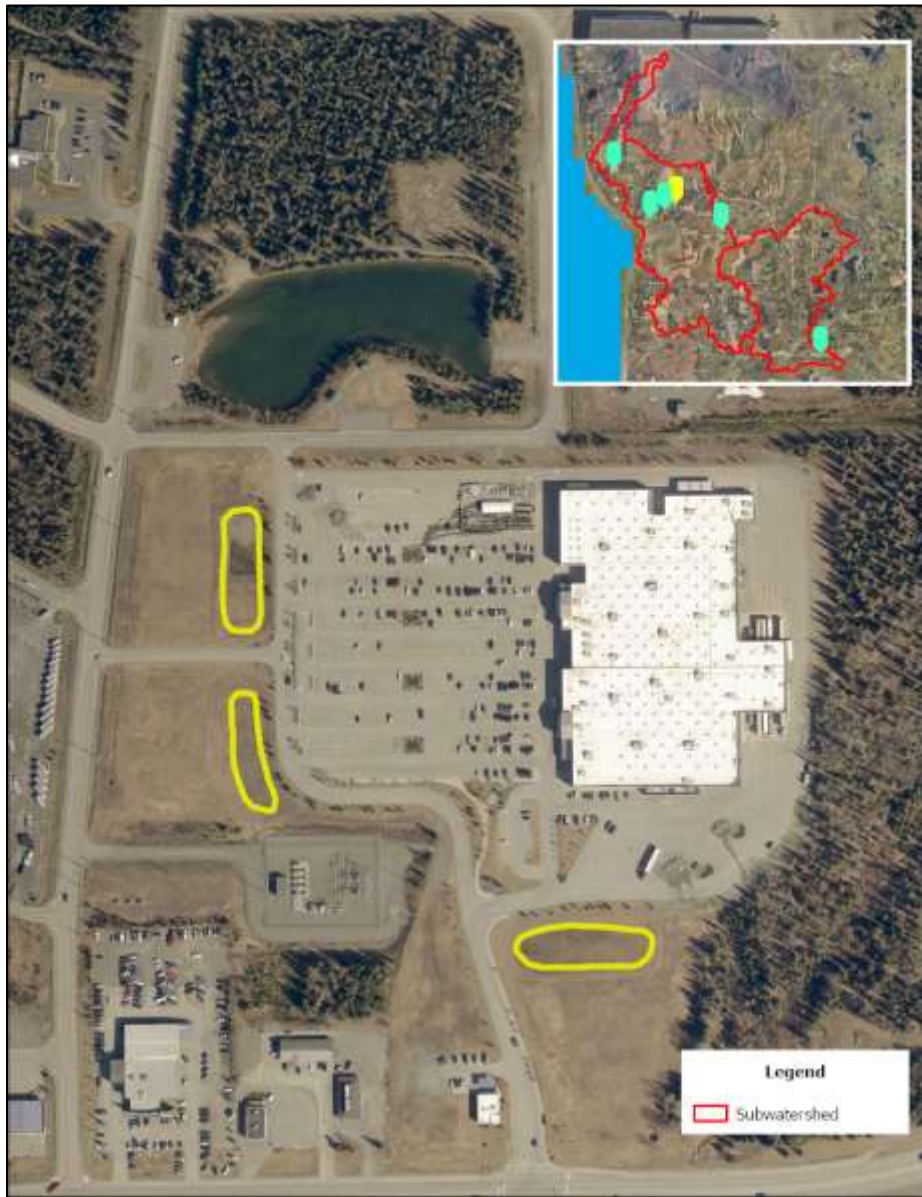
Walmart parking lot. Highlighted in yellow are settling ponds.
